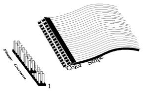
The motherboard supports up to two 720 KB, 1.44 MB, or 2.88 MB 31/2" drives and 360 KB and 1.2 MB 51/4" drives. The connecting cable is a 34-pin ribbon connector with two 34-pin edge connectors for attaching the floppy disk drives. There is a small twist in the cable between the floppy connectors. The last (end) connector should be connected to floppy drive A:.
